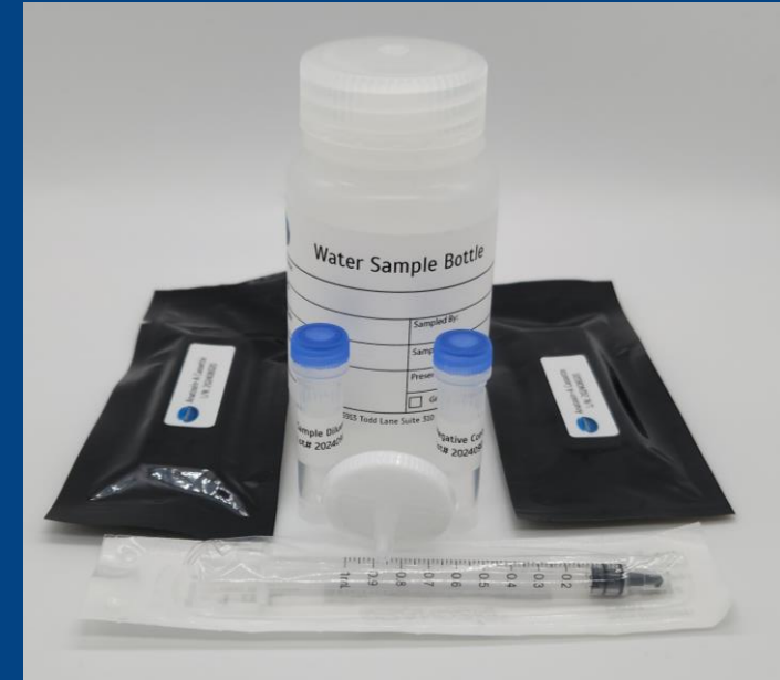
Attogene first of its kind ATX lateral flow based receptor binding assay kit. Cat#AU2062 for recreational water – Field Based.
